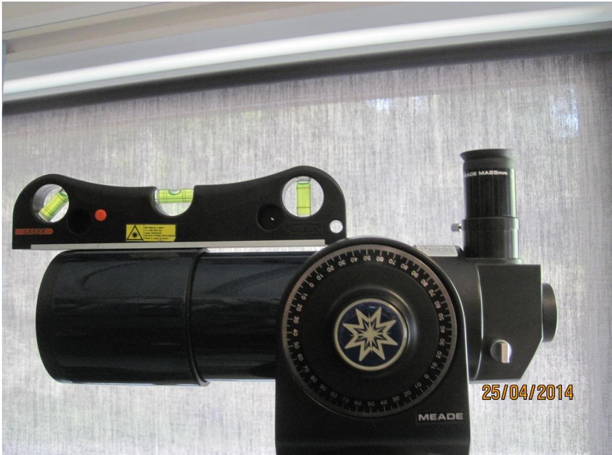
Telescope in “**Home Position**”: tube in the north direction and horizontal plane.
